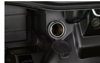
DC power outlet
